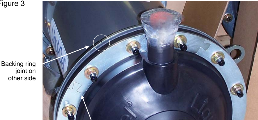
Backing ring joint on this side
