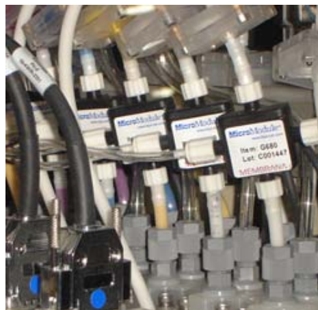
0.5 x 1 SuperPhobic® Contactors Installed on a Wide Format Ink Jet Printer
