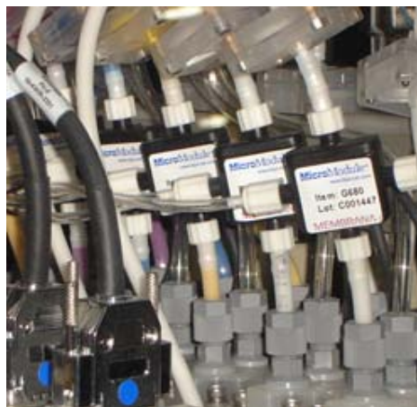
0.5 x 1 SuperPhobic® Contactors Installed on a Wide Format Ink Jet Printer
